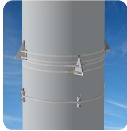
Installation of ice deflectors
